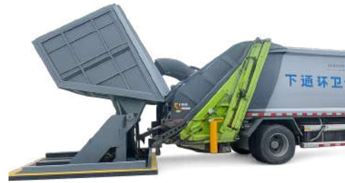
Direct transfer connection between the buried unit and the collection vehicle
